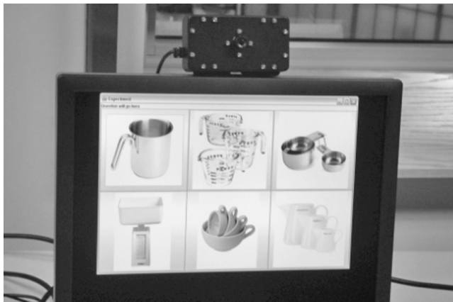
FIGURE 6.5 A small eye contact sensor was mounted on top of the monitor where the cooking tools are displayed to detect whether the participant is looking in the direction of the monitor. (From Torrey et al., 2007.)
